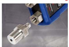
Crystal Pressure Fittings\* are machined in high-strength 316 Stainless Steel to operate at 10 000 psi/700 bar. Removable CPF adapters shift everyday thread wear away from the HPC40 Series' ports, while a self-venting weep hole alerts you before you disconnect from a pressurized system.
