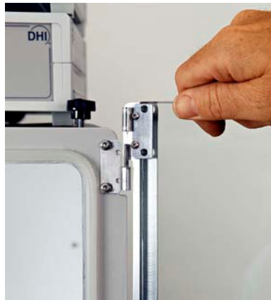
Figure 13. Installation of draft enclosure doors.
