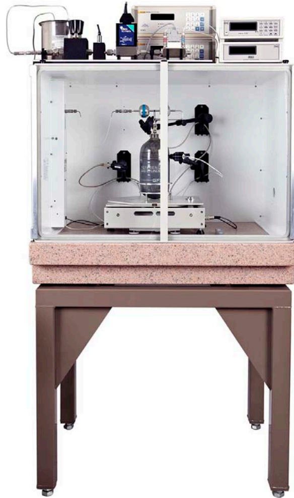
Figure 9. GFS draft enclosure on vibration isolation table
