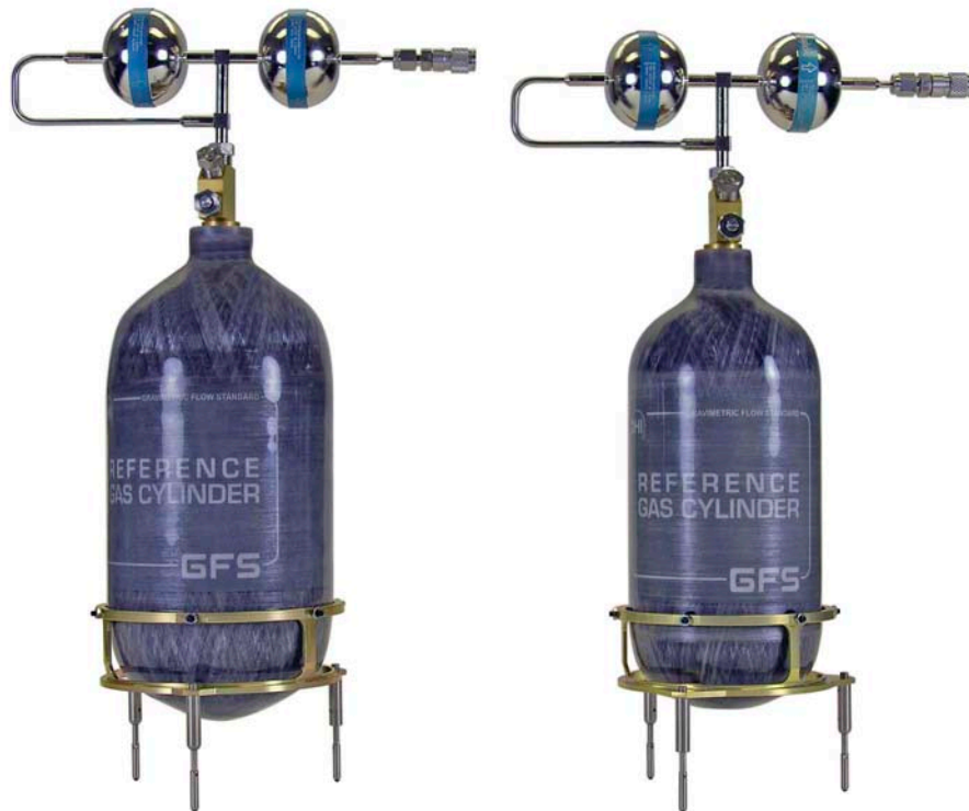
Figure 6. 1.5 liter and 1.1 liter reference gas cylinder assemblies
