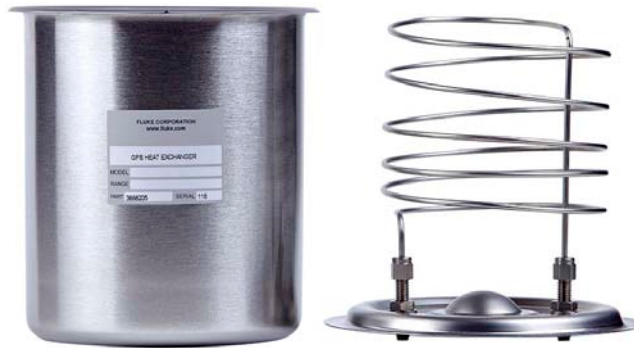
Figure 27. Heat Exchanger unassembled
