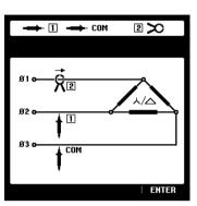
• On screen graphics show you how to set up 3-phase power measurements
