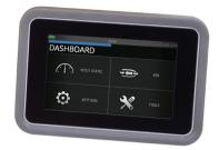
A rechargeable battery pack enables up to eight hours of continuous ADTS Touch wireless use. The battery can be charged by the ADTS Touch when connected to the test set, by power cable, or by an optional desk charger.
