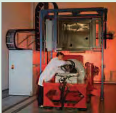
V9mkII shaker with slip-table being set up for testing automotive components.
