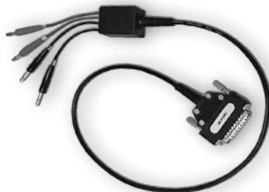
Cable adapter CANON 25-4 x Banana. Four terminal resistance measurement in build-in meter is accessible with the adapter. The option enables also direct measuring of ambient temperature via external RTD temperature sensors.
