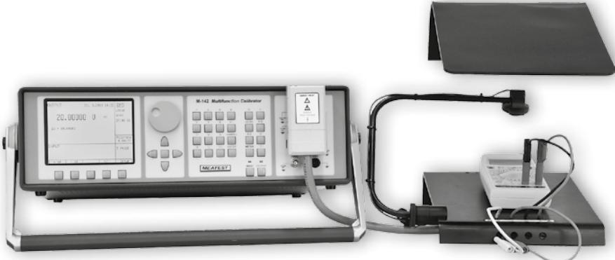
CamOcr camera module extends possibilities of MEATEST automatic calibration software Caliber. CamOcr is designed for scanning of 7 segment digital displays.
