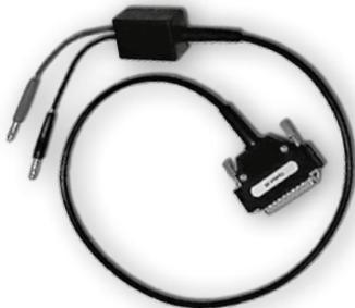
Cable adapter CANON 25-2 x Banana. With the adapter external source of signal can be measured with internal build-in multimeter. Option 40 enables measuring of DC voltage to 12 V, DC current to 25 mA, frequency to 15 kHz and temperature of TC temperature sensors.
