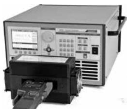
Actively cooled 25-turn current coil for calibration of clamp ammeters up to 3000 A.
