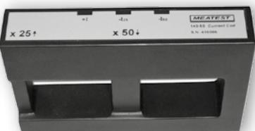
25/50 turns current coil for calibration of clamp ammeters. Maximal range 1500 A.
