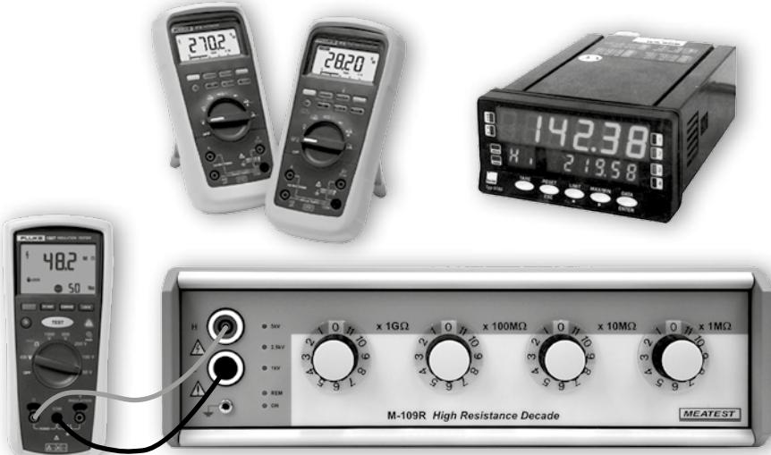
Calibration and verification of resistance meters with test voltage up to 5 kVDC – insulation testers, safety testers, megohmmeters, ...
