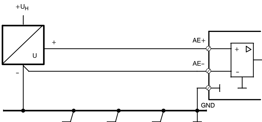
Figure 2-37 Double-pin wiring of a voltage source with positive polarity to ground
