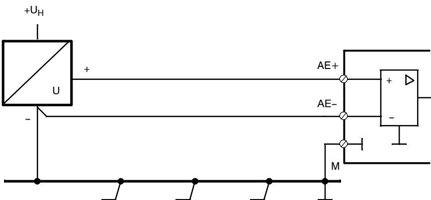
Figure 2-36 Double-pin wiring of a voltage source with negative polarity to ground
