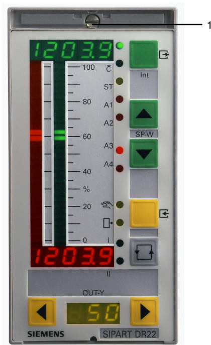
Figure 5-1 Front module with rating plate and cover removed
