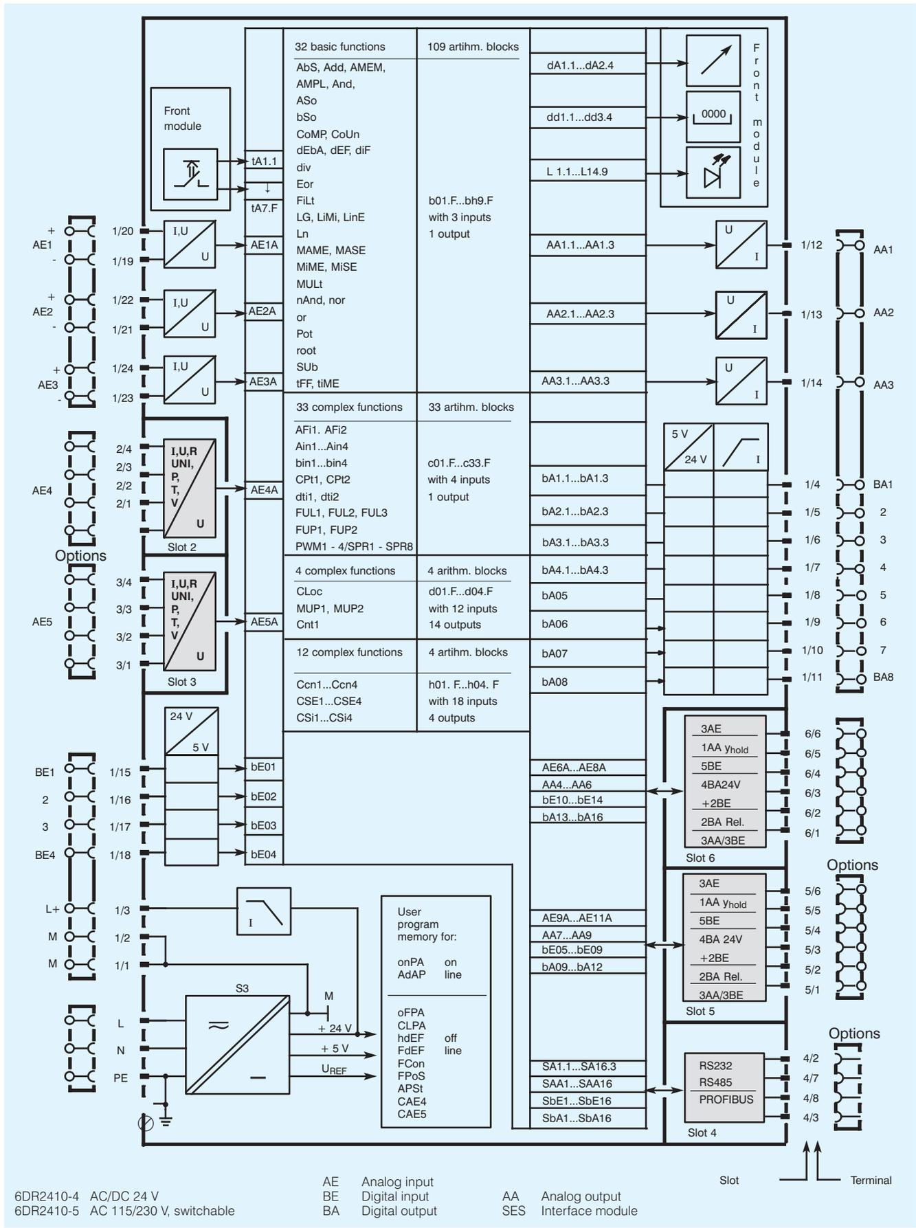
Fig. 7/4 SIPART DR24 multi-function unit, function diagram
