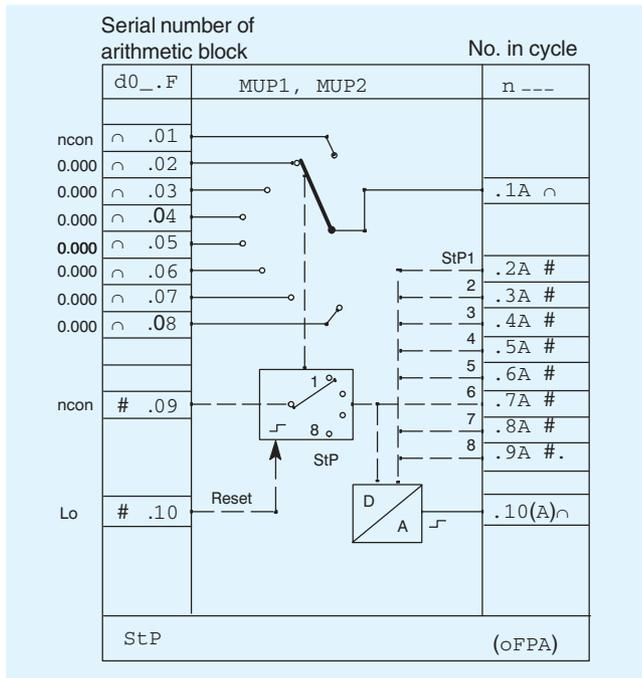
The multiplexer enables up to 8 analog inputs to be switched through to a single output. This switching operation is controlled by the signal on the cycle input d0\*.09 (switch over in a closed ring). Each switching signal is indicated by a Hi signal on a separate output. These signals can, for example, be connected to the programmer's inputs to select a particular program. In addition, the current position can be displayed by connecting the d0\*.10 output to the digital display dd3.
