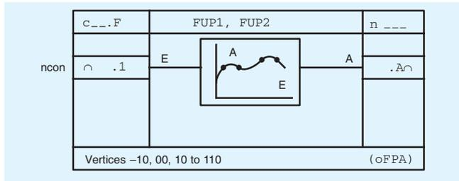
Curve calculator with 13 vertices between -10 and +110 % of the input signal range:
