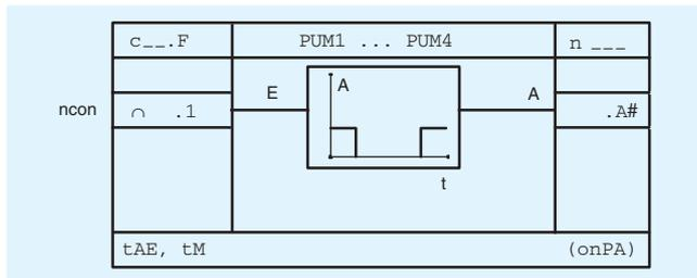
The pulse-modulator converts an analog signal into a pulse-width-modulated binary signal.
