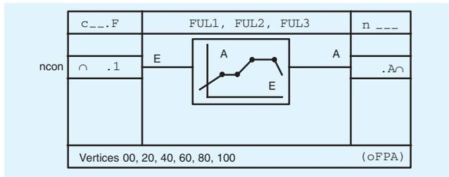
Curve calculator with 6 vertices between 0 and 100 % of the input signal range.
