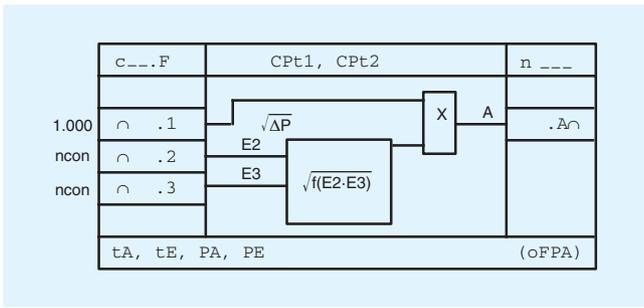
Correction computers are used to calculate the rate of flow of gases from the differential pressure  $p$ , correcting for fluctuations in pressure and temperature. Mass flow and volume flow based on the operational state can be corrected, as well as volume
