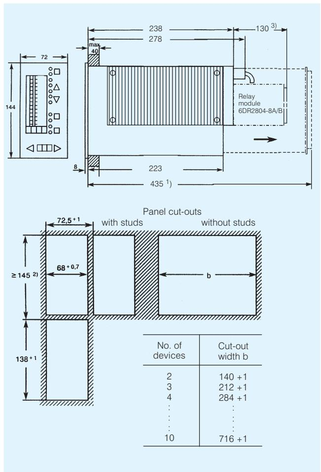
1) Space required for removal of main circuit board.
