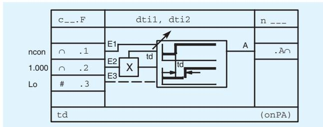
Output = input offset by time *t<sub>d</sub>*:
