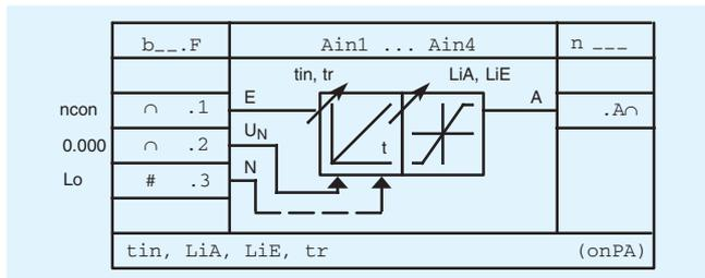
The analog variable on input .1 is integrated.
