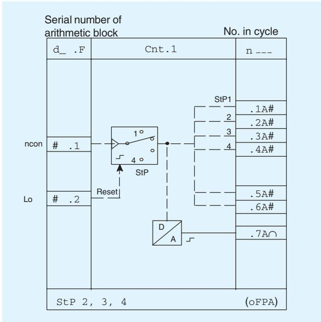
The demultiplexer is primarily used for switching over the display and control elements (multiple controller, max. 49).
