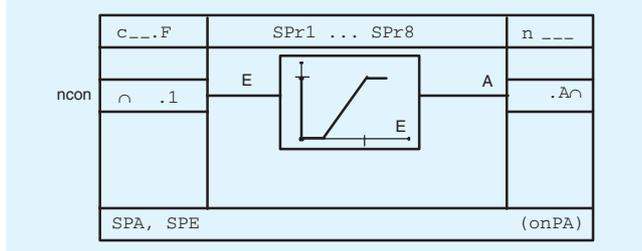
The split range function comprises a straight-line equation between the base point SPA (output value 0) and the turning point SPE (output value 1).
