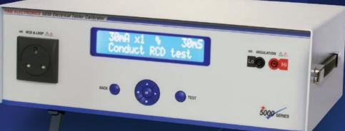
A precision instrument designed to calibrate RCD, loop, insulation, earth testers and multifunction installation testers. The 5030 accurately simulates RCD trip times and measures currents produced by RCD testers. It replicates loop impedance and auto adjusts for local line impedance. It also provides insulation resistances and measures test voltages and currents.
